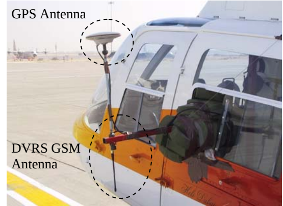
Fig. 1 System installation for the helicopter test
