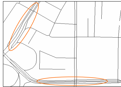
Figure 9 Undetected mismatches in parallel lanes
